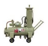
The Hilco Coalescer/Separator, available in stand-alone or portable models, removes moisture and particulate contamination from steam and gas turbine lube oils. For more information, request brochure HSS-1.
